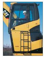
**Fixed Cab Riser.** The fixed cab riser offers a very stable and comfortable method to raise the cab by 1200 mm to offer better viewing around the machine. Well positioned steps lead up to the cab from the ground level. Fixed cab riser option is only available for the M322D MH.
