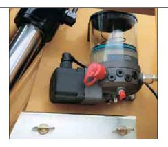
**New Auto-Lube System.** The new automatic lubrication system provides the optimal amount of grease to all the main lubrication points, including the bucket linkage. The lubrication interval can be adjusted through the monitor, and status messages for the auto-lube system are displayed.
