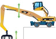
SmartBoom. It allows the operator to fully concentrate on production. The unique Cat SmartBoom significantly enhances operator comfort and job efficiency. Loading is more productive and more fuel efficient as the return cycle is reduced while the boom down function does not require pump flow.
