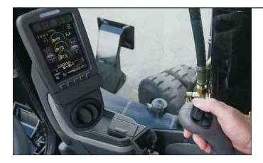
**Tool Control.** Ten hydraulic pump flow and pressure settings can be preset within the monitor, eliminating the need to adjust the hydraulics each time a tool is changed. Selecting the proper setting from the monitor menu instantly provides the operator with the correct amount of flow and pressure for the tool.
