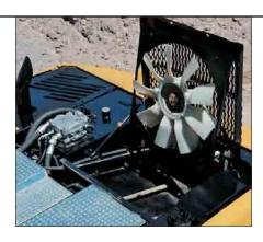
**Easy to Clean Coolers.** Flat fins on all coolers reduce clogging, making it easier to remove debris. The main cooling fan and air conditioner condenser are both hinged for easier cleaning.
