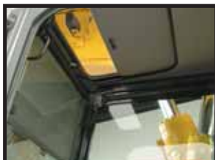
Large sun roof with integrated sun shade
