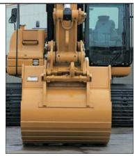
**Bucket Linkage.** Two bucket linkages (DB and TB) are available, with lifting eye on the power link.
