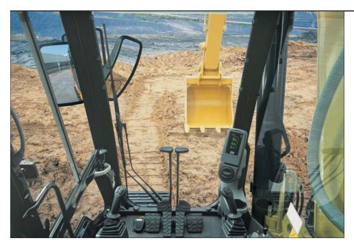
**Operator Station.** Thanks to its higher position, the 336D HDHW cab gives the operator an enhanced view over the trench, the truck or the crusher. The workstation is spacious, quiet and comfortable, assuring high productivity during a long workday. The air conditioner and attachment switches are conveniently located on the right-hand wall, and the key switch and throttle dial are on the right-hand console. The monitor is easy to see and maximizes visibility.
