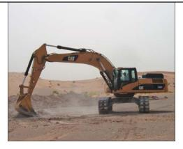
**HDHW Undercarriage.** The wide and durable Cat undercarriage absorbs stresses and provides excellent stability. Additionally, the high ground clearance is ideal in rocky environments, bringing the upper frame in a safer high position.
