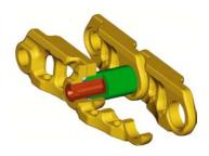
**Tracks.** The 336D HDHW comes standard with grease lubricated tracks. The track links are assembled and sealed with grease to decrease internal bushing wear, reduce travel noise and extend service life lowering operating costs.
