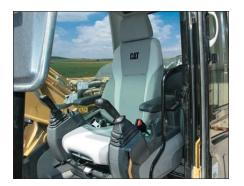
**Adjustable Consoles.** Redesigned consoles feature a simple, functional design to reduce operator fatigue, ease of switch operation and excellent visibility. Both consoles have attached armrests with height adjustments.
