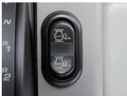
The electric throttle control allows the operator to perfectly match the engine speed to working conditions
